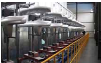
↑ Caldan P&F100 floor conveyor - operating in China - surface treatment of auto bumpers
