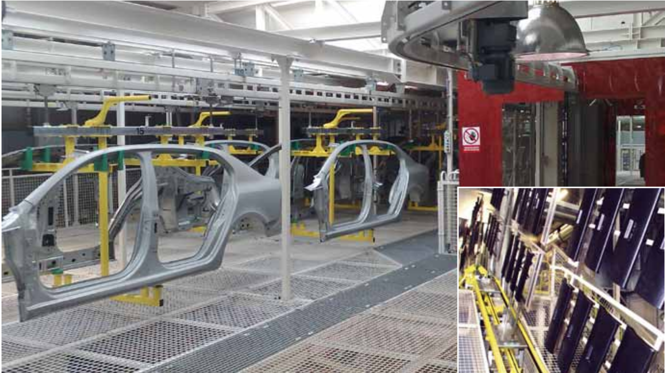
↑ Caldan P&F400 overhead conveyor - operating in Europe - transportation of auto body parts
