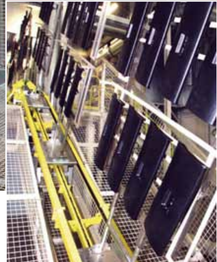
↑ Caldan HD100 floor conveyor - operating in Germany - surface treatment of auto parts, interior
