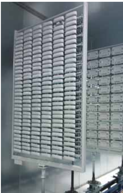
↑ Caldán P&F100, power & free floor conveyor, operating in the UK; surface treatment of plastic components, automotive industry
