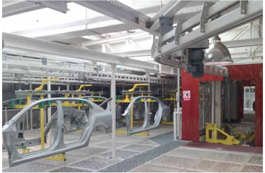
↑ Caldán P&F400, power & free overhead conveyor, operating in Europe; transportation of auto body parts
