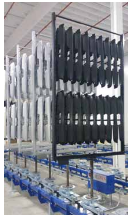
↑ Caldán P&F100, power & free floor conveyor, operating in USA; surface treatment of plastic components, automotive industry
