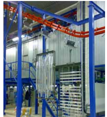
↑ Caldán P&F400, power & free overhead conveyor - operating in Germany - surface treatment of various components, automotive industry
