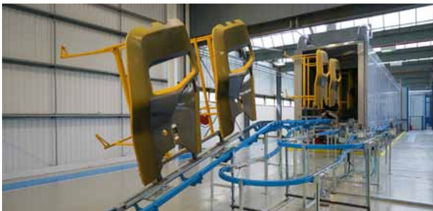
↑ New Caldán P&F140, heavy duty power & free floor conveyor - operating in the UK - surface treatment of plastic components, automotive industry
