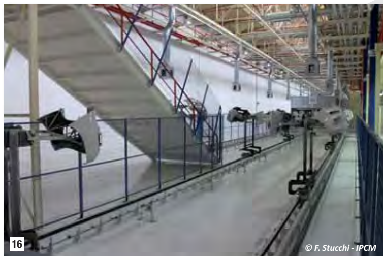
16 The finished bumpers leaving the final oven.
