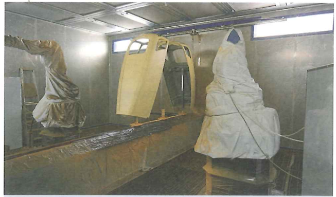
Parts up to 3000 mm long and 2000 mm high can be painted in the booth.
