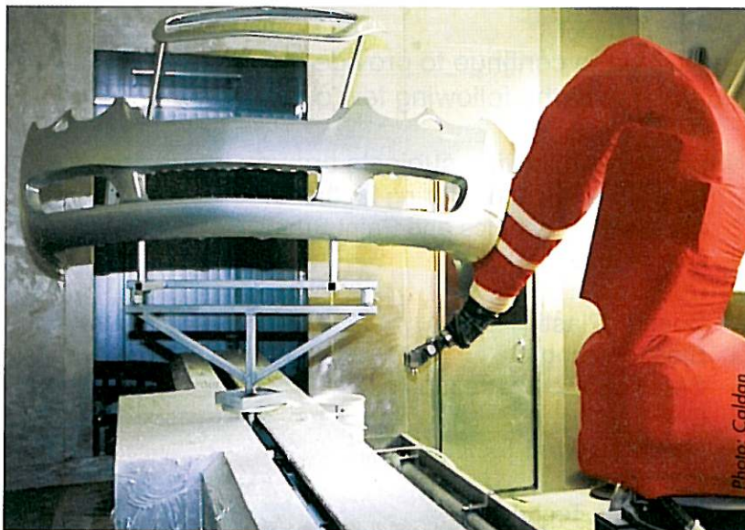
Product carrier with set of vehicle parts in the coating booth. The conveyor allows the exact positioning necessary for robot application, even with large parts.
