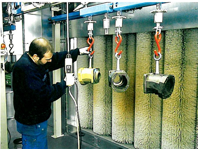
At the company Brüninghaus, the crossbeams have different pivotal links for large and small parts. The picture shows the conveyors with the pivotal links in front of the spray wall.
