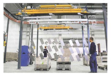
◀ ▲ The new conveyor technology allows workpieces of different shapes and sizes to be conveyed.
