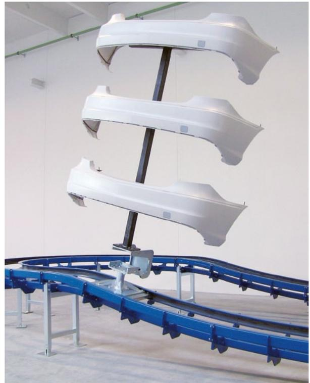
The floor conveyor, shown here in the manufacturer's testing centre, exploits the benefits of conventional power & free systems, thus making it highly flexible.
