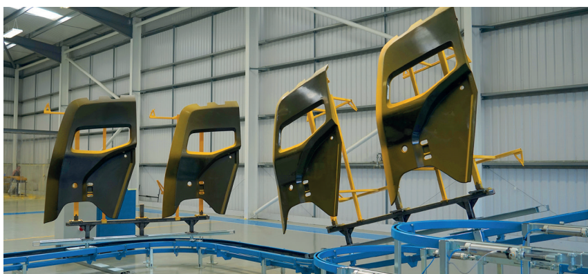
↑ New Caldán P&F140, heavy duty power & free floor conveyor - operating in the UK - surface treatment of plastic components for the automotive industry
