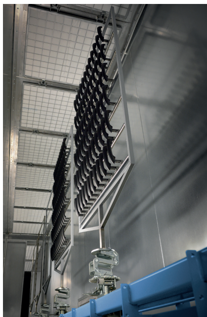
↑ Caldan P&F120, power & free floor conveyor - operating in Poland - surface treatment of plastic parts for automotive locking systems
