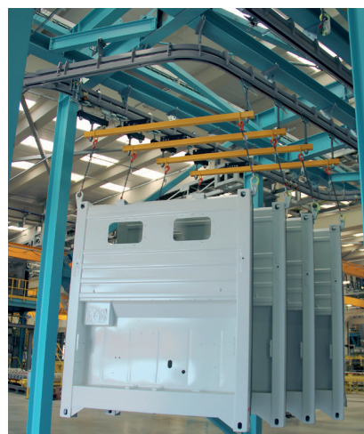
↑ Caldan P&F400, power & free overhead conveyor - operating in Chile - surface treatment of container frames, doors & back-covers
