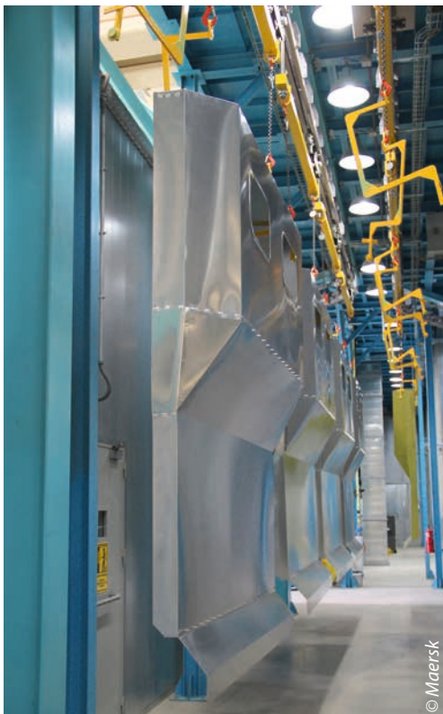
Raw material and interim buffer zones are arranged in parallel on the painting line.
