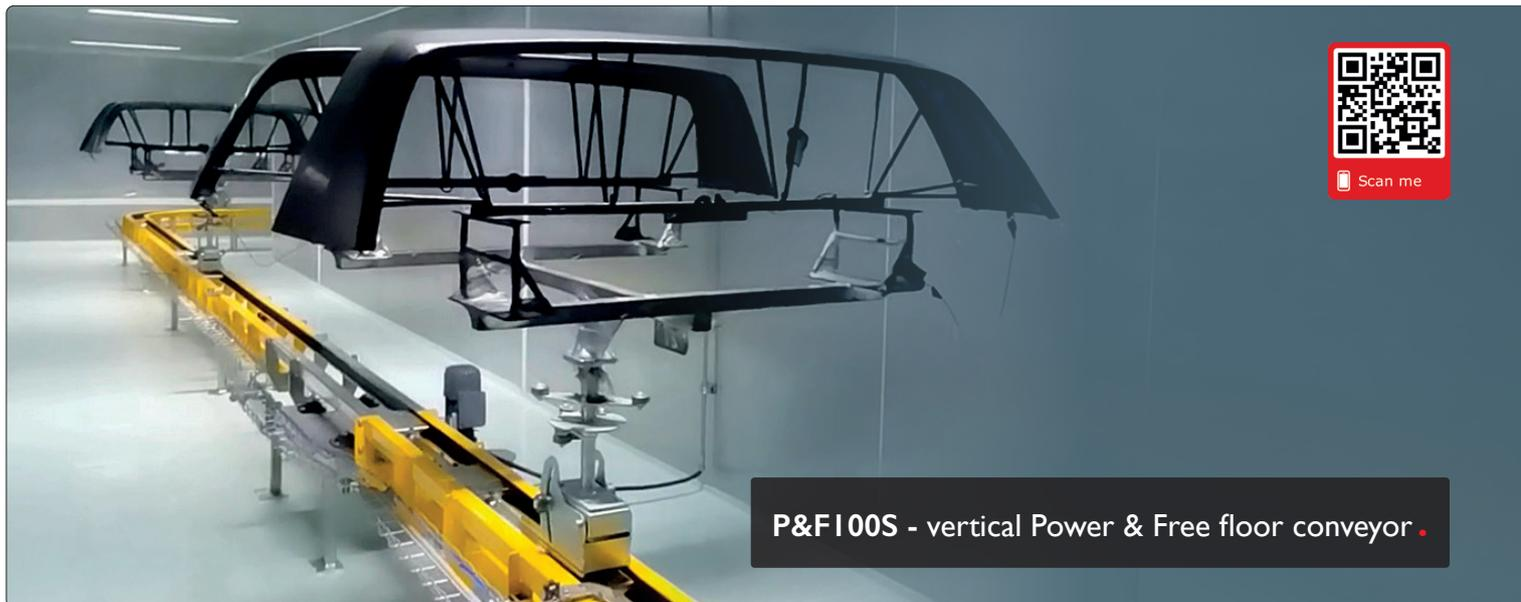
**P&F100S - vertical Power & Free floor conveyor .****P&F100S****CONVOYEUR AU SOL - POWER & FREE**
