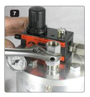
Fasten ball valve with wrench. Mounting hole for lever pointing towards operator.
