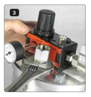
Unfasten the ball valve with the wrench (counter clock-wise).
