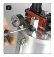
Unfasten screw in the lever on the original ball valve (to be re-used).
