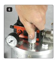
Fasten ball valve in container (clock-wise).
